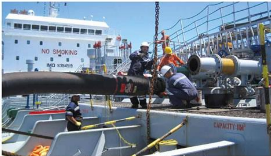
Trelleborg's new hose seen being connected during an STS
