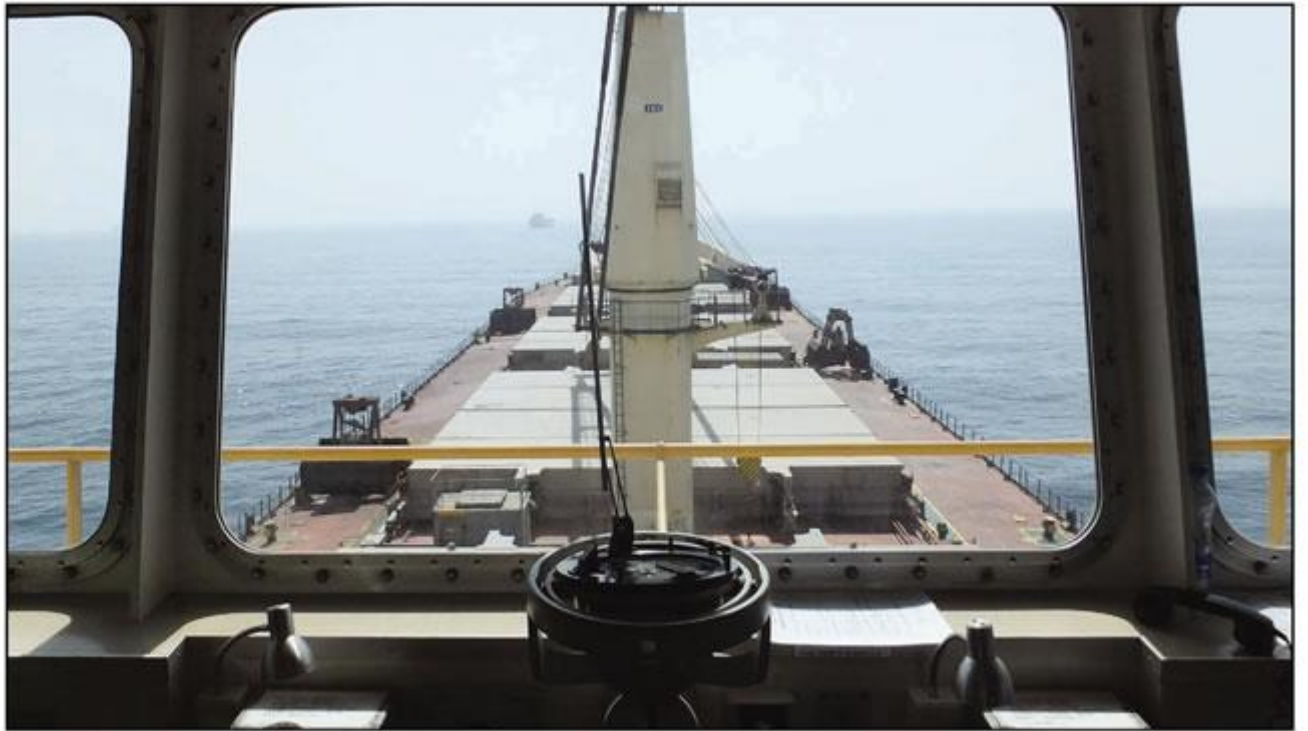
Figure 2: View from the bridge over the centreline gyro repeater
