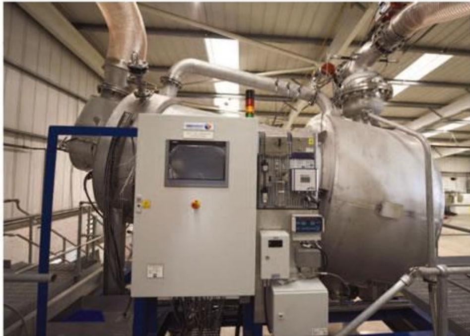
Sea Guardian Inert Gas Generators' gas output is linked to specially designed Gas Lift Diffusion (GLD) pipe assemblies mounted inside the ships ballast tanks.
