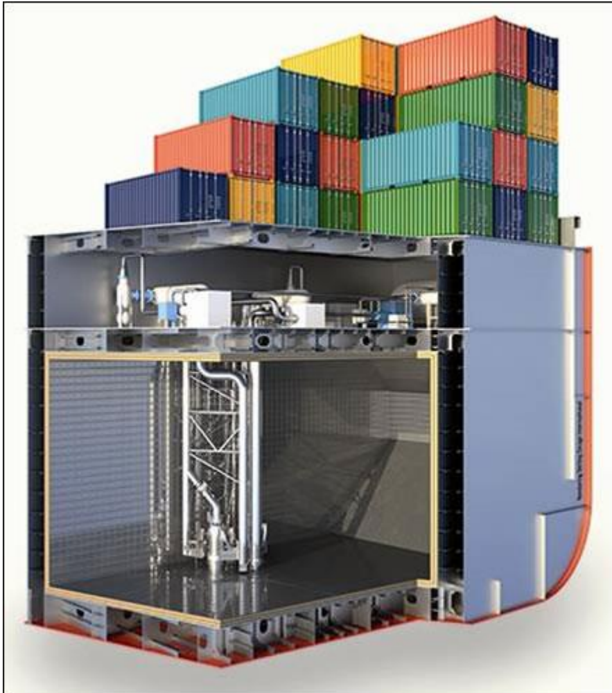
Design of a fuel tank for a container ship. (Graphic: © GTT)
