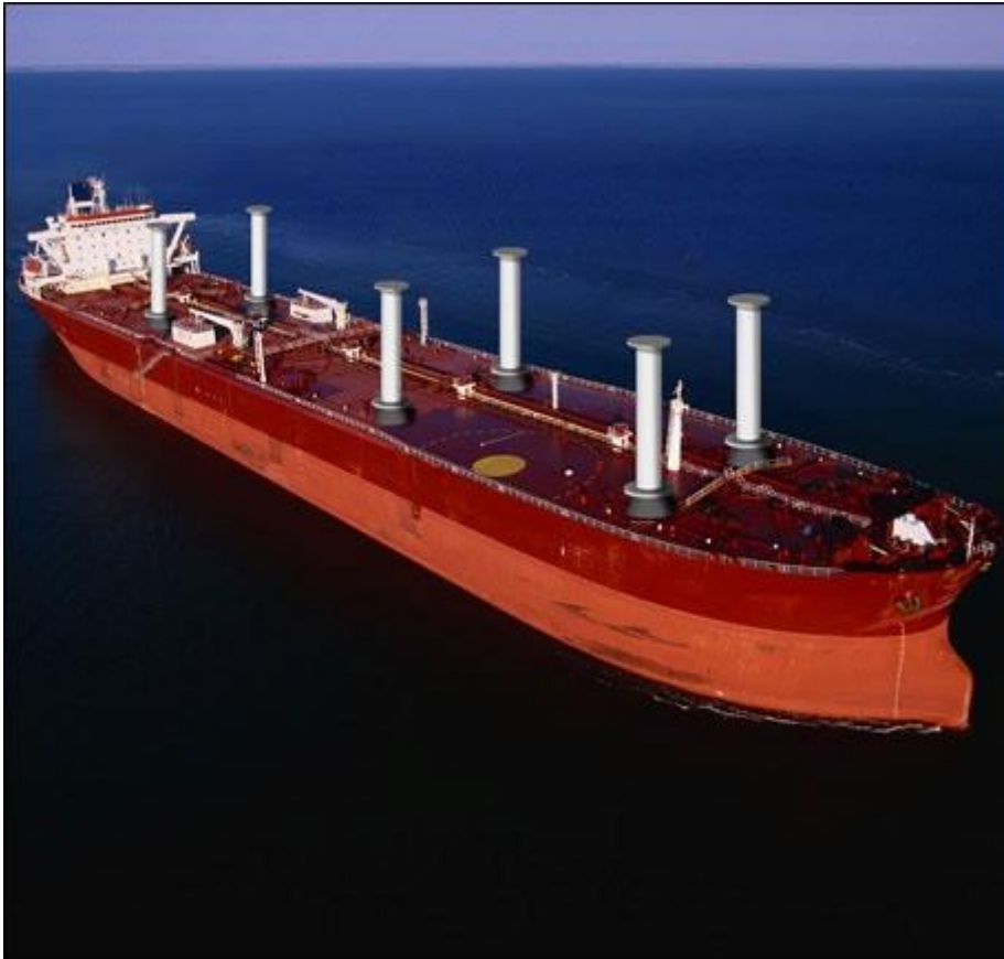
Example of a vessel-specific installation of six Norsepower Rotor Sails on a tanker vessel.
