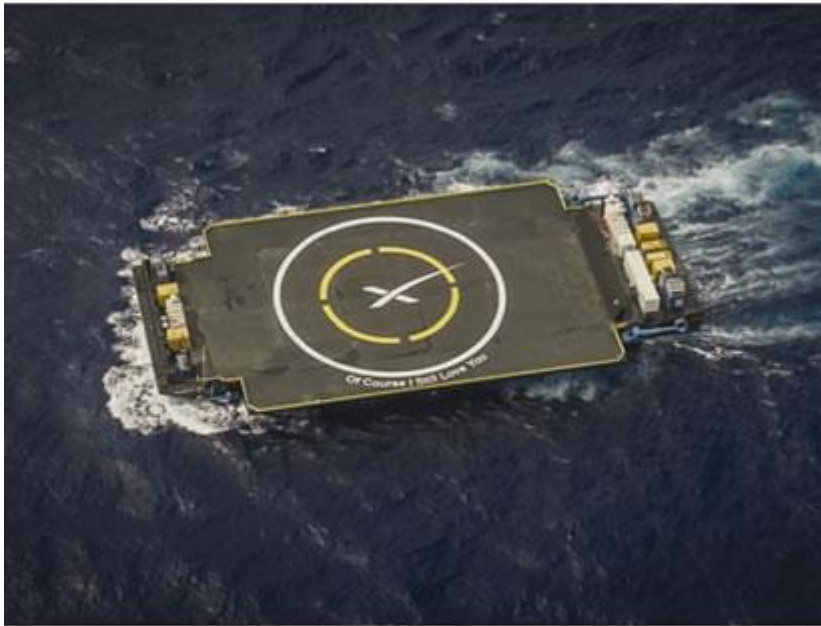
SpaceX has already created its own drone ship to use as a landing platform for its launch vehicles, constructed from a converted barge
