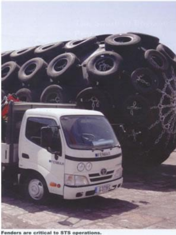
Fenders are critical to STS operations.
