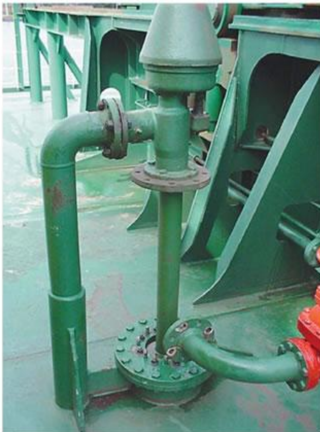
Hold cleaning equipment in the stowed position above the deck. Note the flange on the deck wash line
