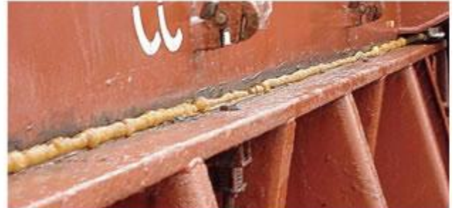
Do not use foam to seal hatches
