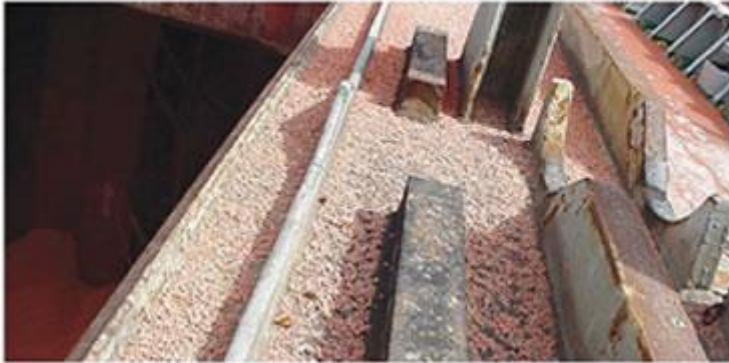
Coaming/trackway covered in fertiliser; below, ship's main deck covered by previous cargo
