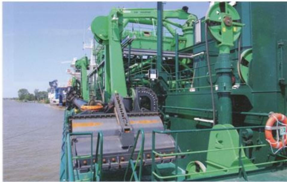
A submersible pump is mounted on the suction pipe to achieve high dredging depths
