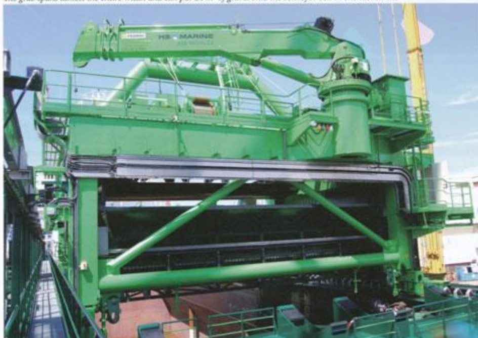
The grab spans almost the entire width and can put 24 m 3 of gravel onto the conveyor belt in one movement
