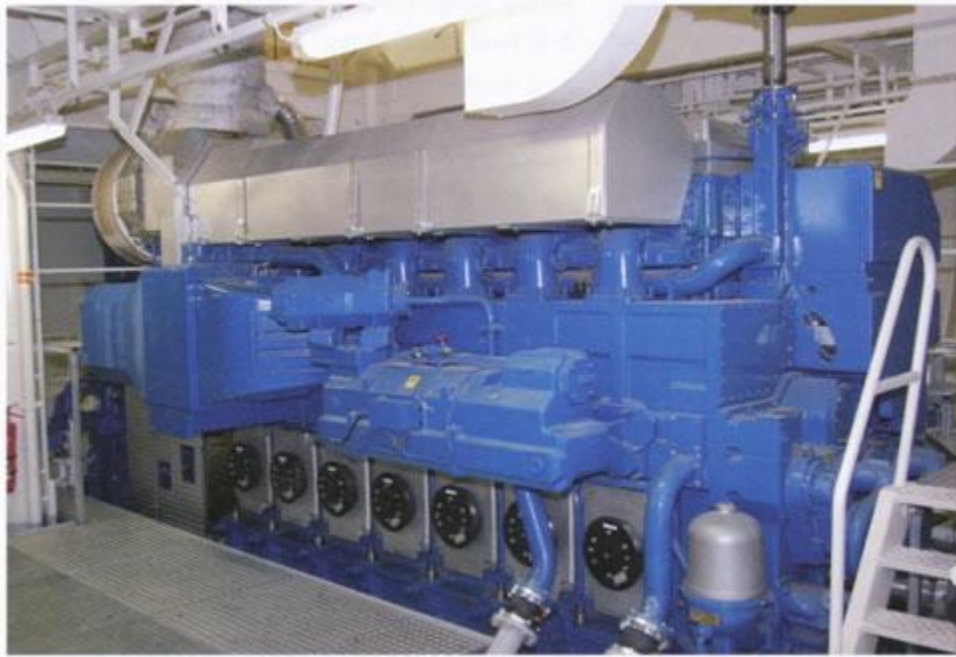
The propellers are driven directly by a pair of Wärtsilä main engines
