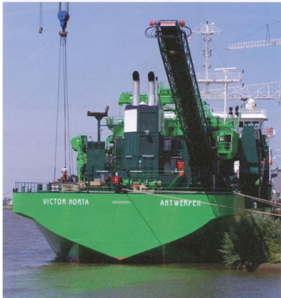
With the dry unloading system, the hold can be emptied in 4.5 hours
