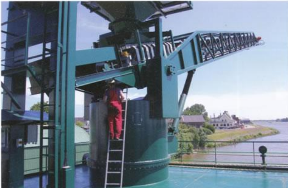
The last part of the conveyor belt system can be swivelled to the correct position
