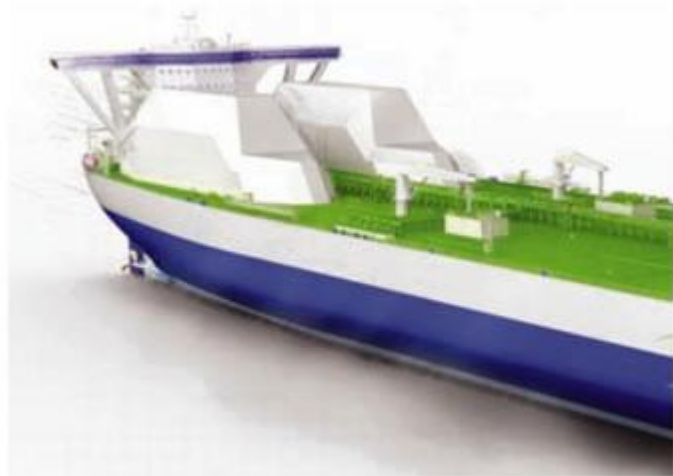
Two gas tanks are fitted on the deck ahead of the accommodation block.
