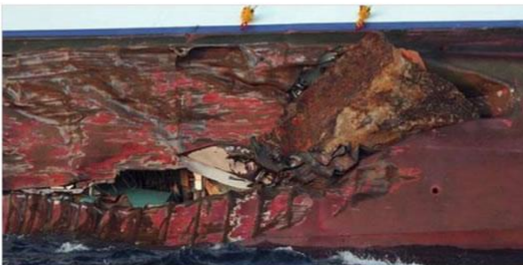
Piece of rock sticking in the damaged Portside hull of the vessel
