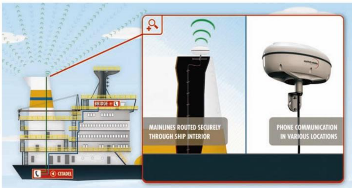
A small, hidden communications terminal with a battery power source could allow crews to stay in contact with shore from a safe room
