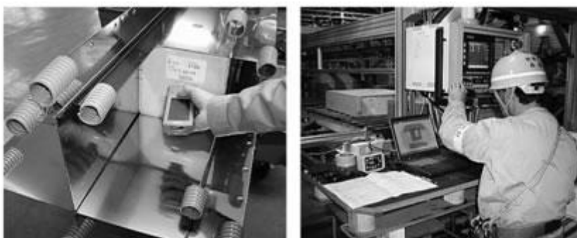
Fig. 9 Logistics and quality control system: LOGIQ for components of cargo containment system (Reading of bar codes on parts and control of resin ropes)
